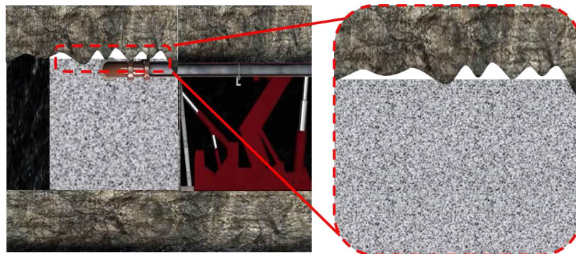
Figure 2. Gaps occurring in paste backfill roof contact
